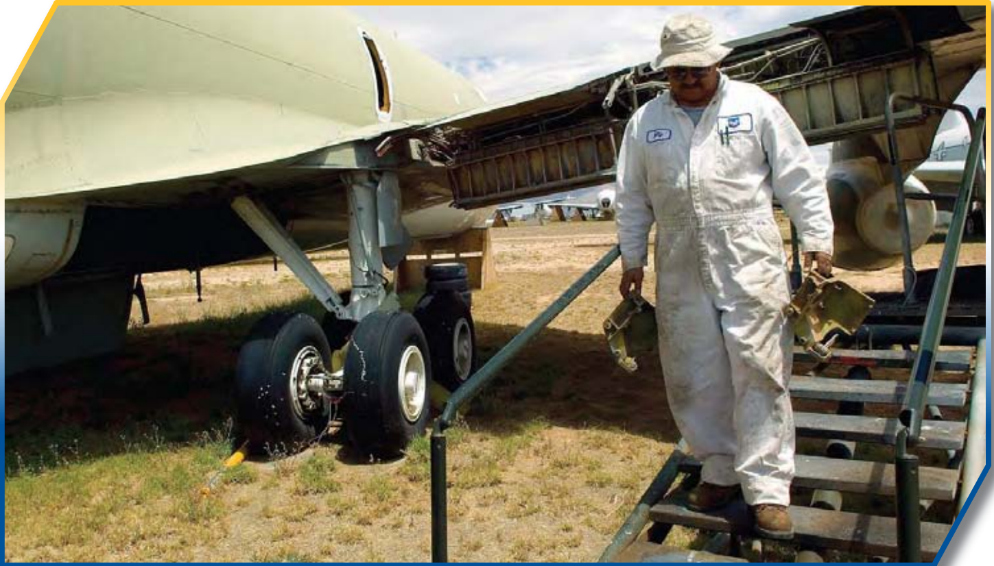
An aircraft mechanic removes support brackets from the wings of a preserved KC-135E Stratotanker at the AMARG storage site at Davis-Monthan AFB, AZ. The brackets will be shipped to Tinker AFB, OK, where they will be used to bring a broken KC-135R back to flying status. The center provides customer services including aircraft regeneration restoring aircraft to flying status, limited depot-level maintenance, parts reclamation, historic storage and disposal functions. (U.S. Air Force photo by Bennie J. Davis III)
