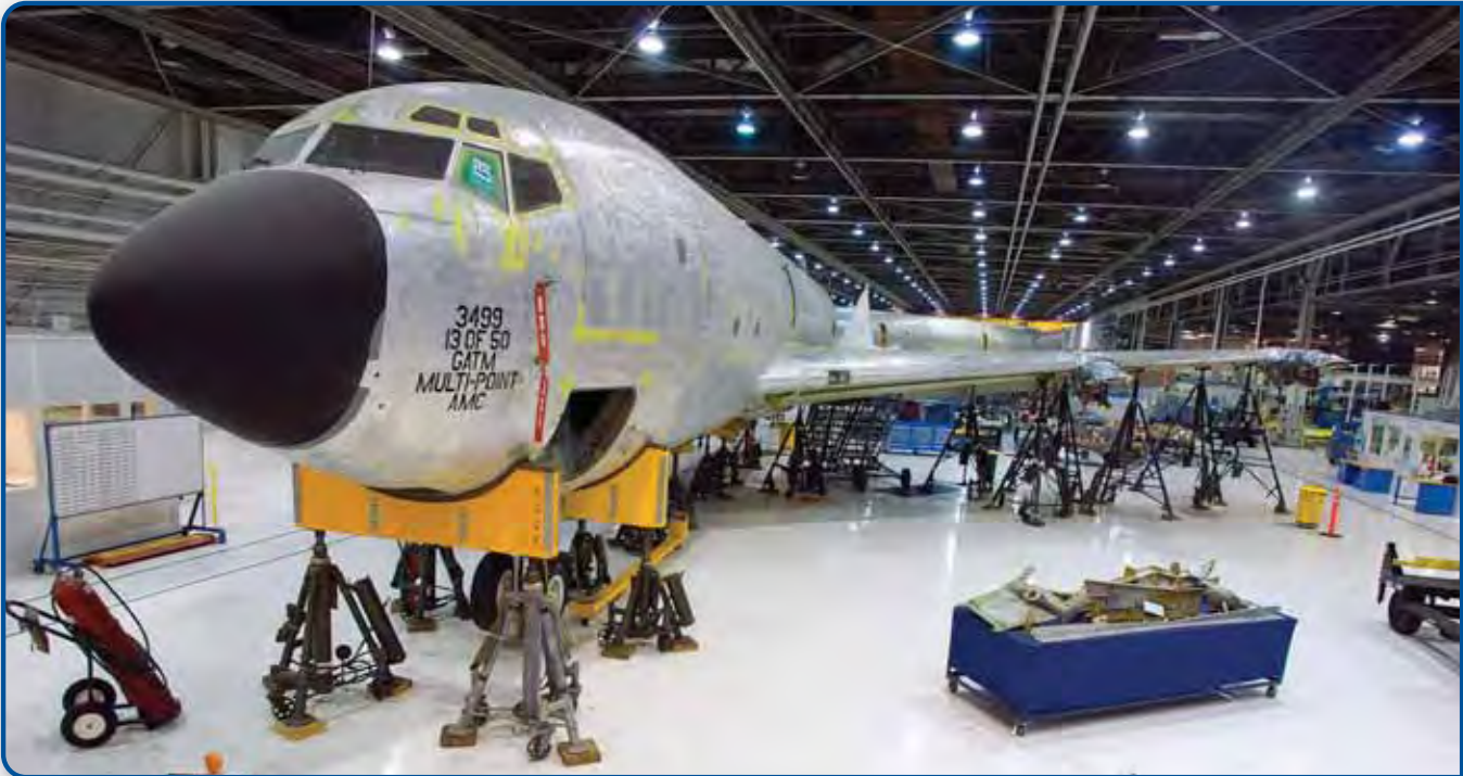
A KC-135R Stratotanker sits inside the Oklahoma Air Logistics Center, Okla., waiting for a full maintenance overhaul. The Oklahoma Air Logistics Center is the worldwide manager for a wide range of aircraft, engines, software, avionics and accessories components.
